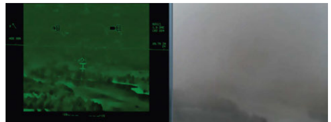
Figure 11: EFVS can increase situational awareness at night and during low-visibility weather conditions.
